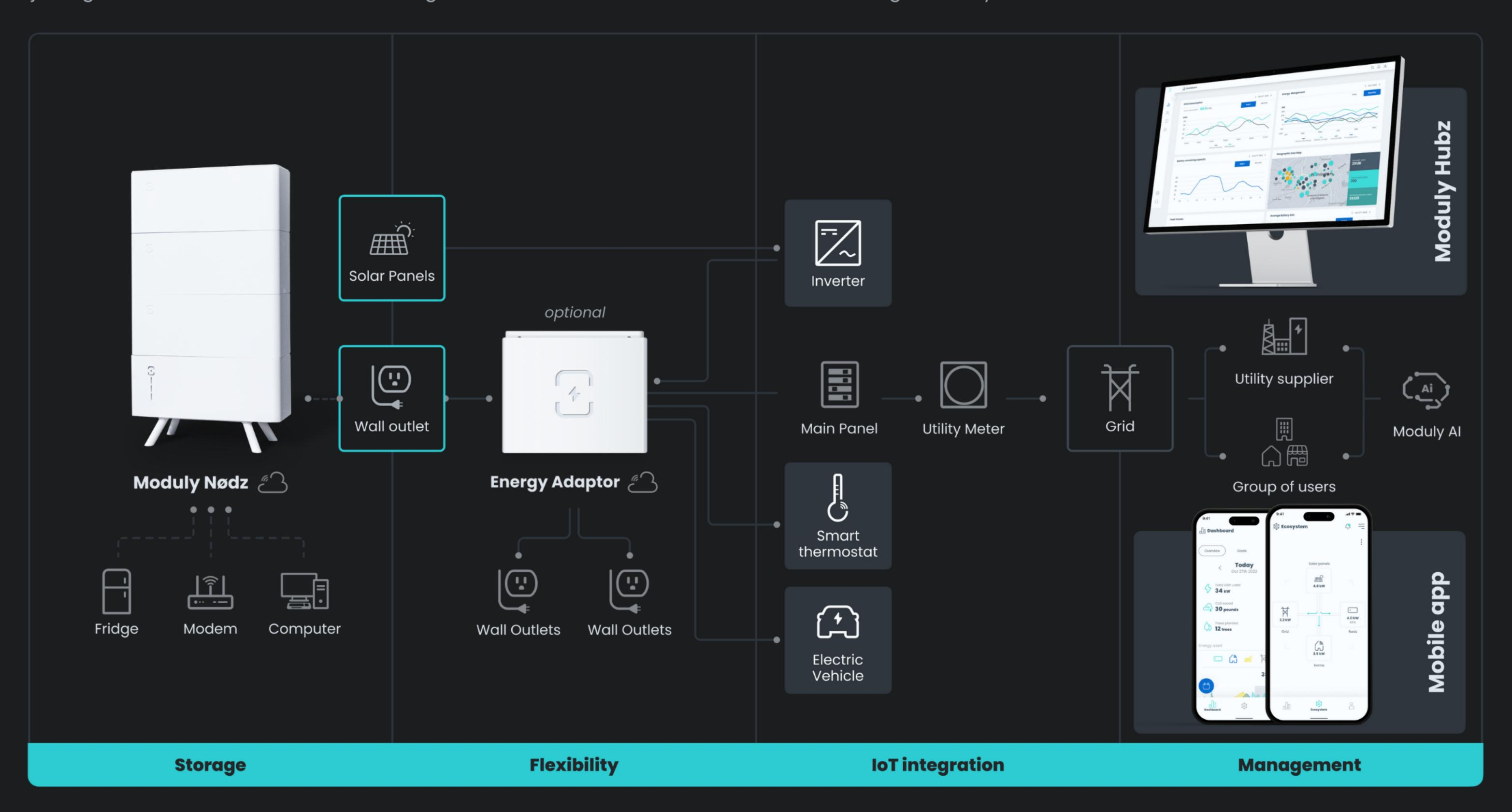
Nødz energy storage performs peak shaving and valley filling while providing resilience onboard. The Adaptor isolates and optimizes the most important circuits during a power outage.
